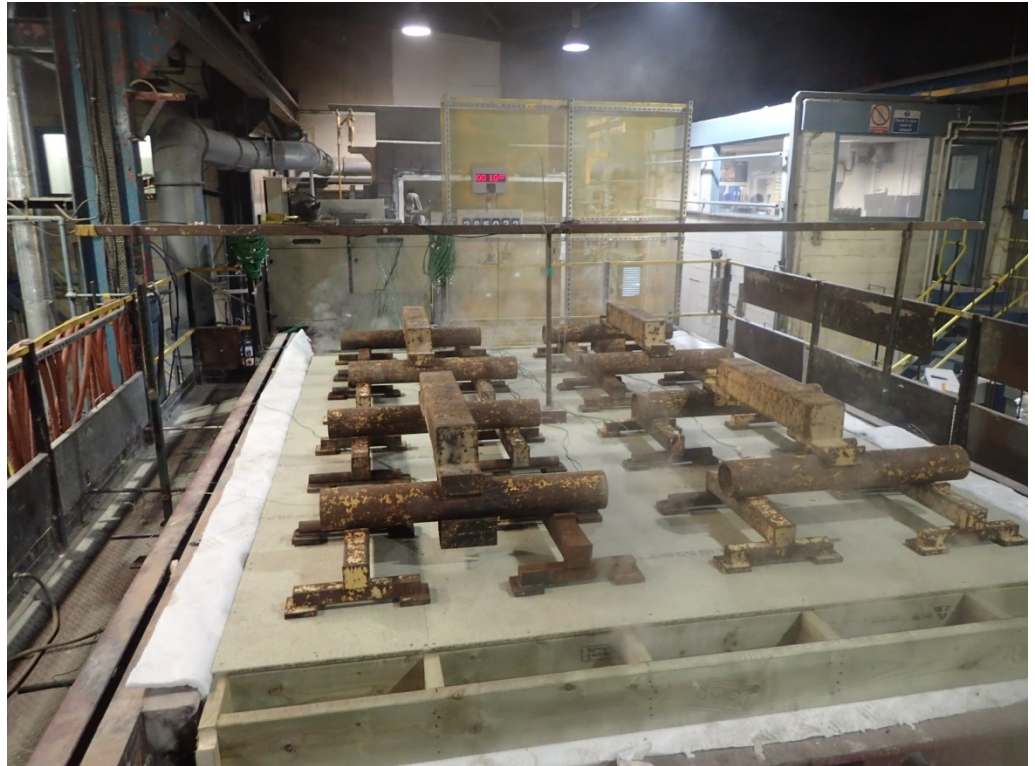
The unexposed face of the assembly after 10 minutes of testing
