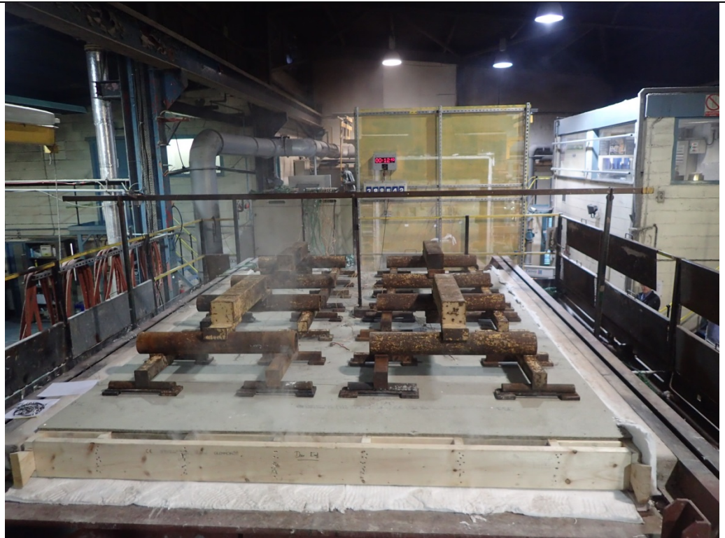
The unexposed face for the assembly after a test duration of 12 minutes
